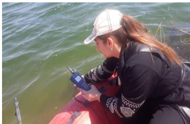
Figure 2. The process of measuring water temperature in an ES 300 apparatus.
